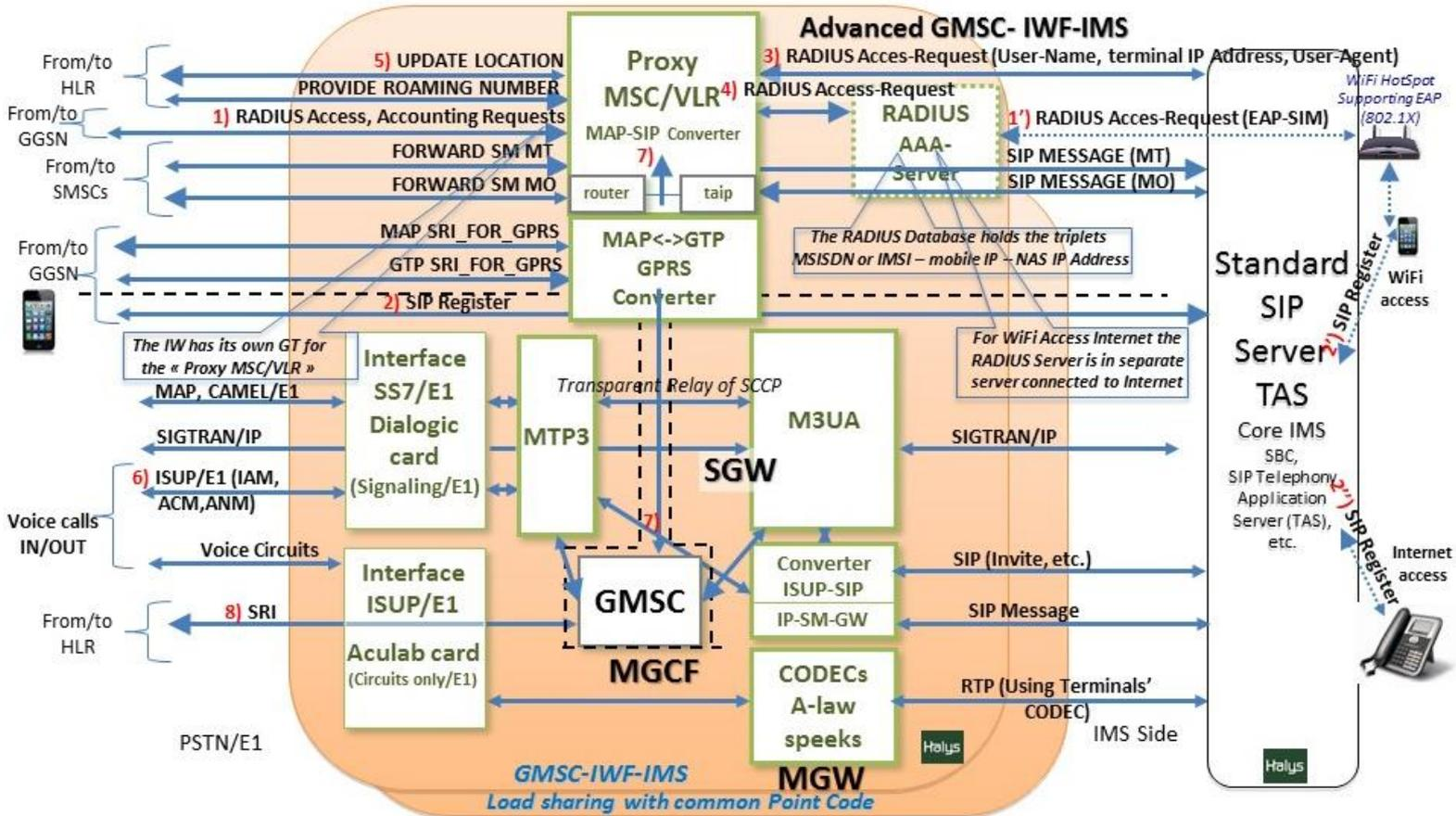
Fig 1 Architecture of Standard GMSC with advanced IWF for IMS fix and mobile terminals (Voice and SMS)
